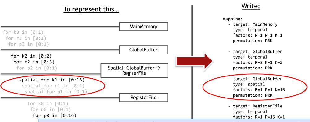
By convention, a block of spatial\_for loops representing a spatial famout from storage level *Outer* to storage level *Inner* are described as a spatial mapping directive targeted at level *Outer*.
